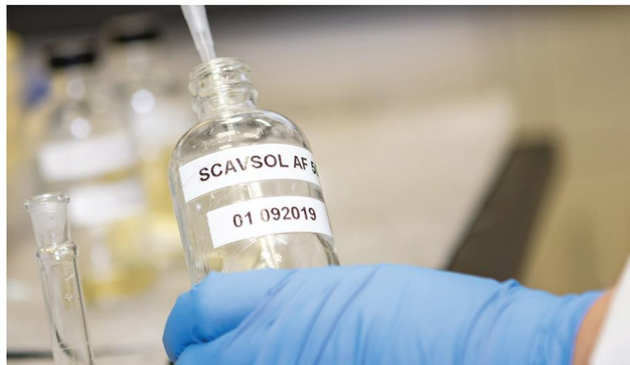
ScavSol AF 50 is an iron chelation technology that controls iron precipitation in the presence of chlorine dioxide. Though a common application in oilfield water sterilization, chlorine dioxide often leads to unwanted precipitation that causes assets to foul, scale and corrode. ScavSol AF 50 can be used to chelate iron prior to chlorine dioxide application and then remain chelated as the product does not allow iron to precipitate.
